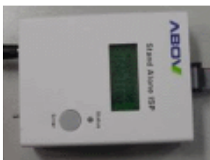
Figure 1-3 StandAlone ISP (VDD power is not supplied)
