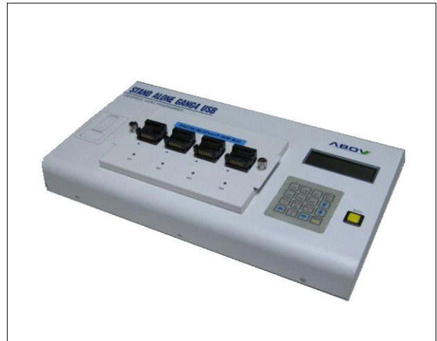
Figure 1-3 Stand Alone Gang4 USB (Gang Writer)
